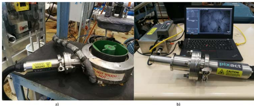
Fig. 1. Mark reactor (a) and bubble measurement (b) used in the laboratory delignification.
