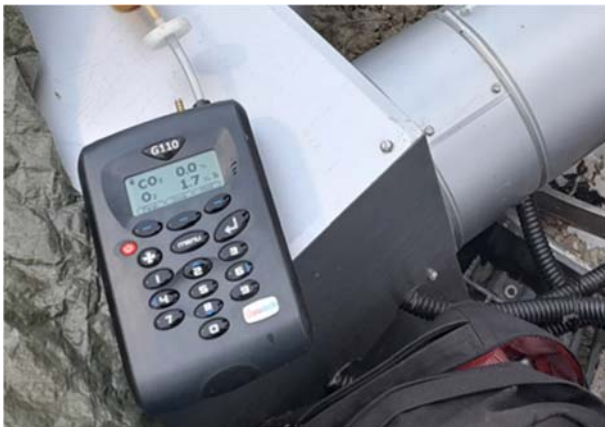
Figure 4. The oxygen content of the residual gas in the top of reactor 2 was nearly zero.
