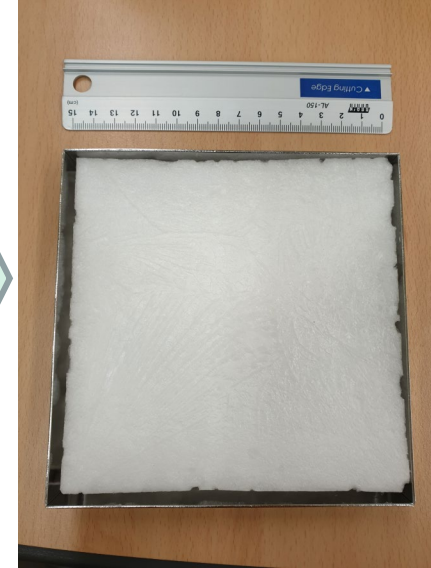
1% dispersion and aerogel for composite
