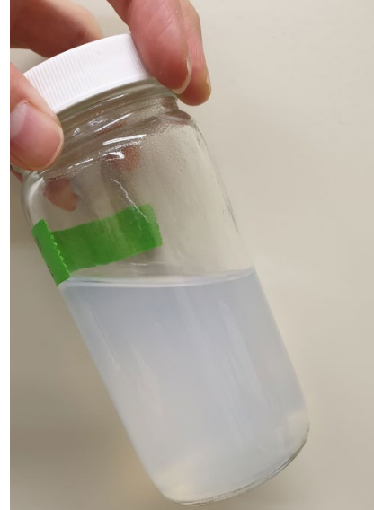
1% dispersion and aerogel for composite
