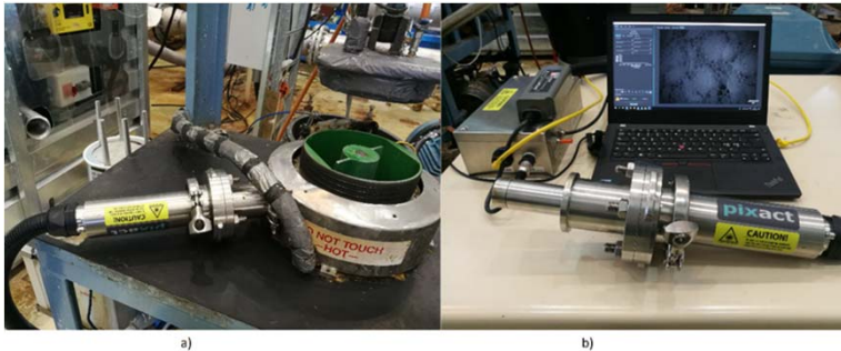
Mark reactor (a) and bubble size measurement (b) used in the laboratory delignification.
